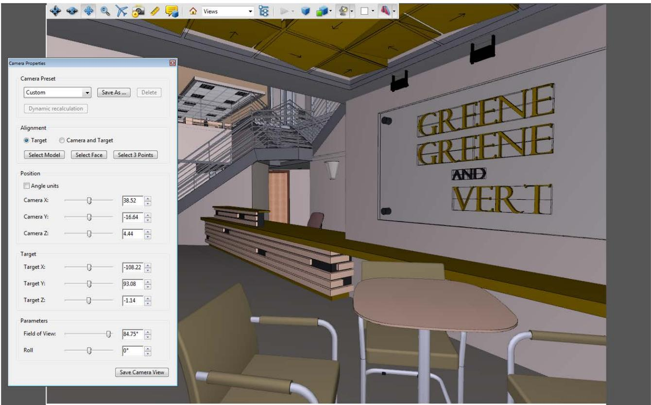
**Image 15:** Creating an interior view and adjusting the camera properties
