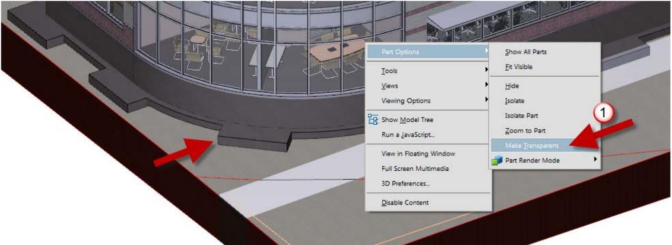
**Image 14:** Making the ground transparent so the footings are visible
