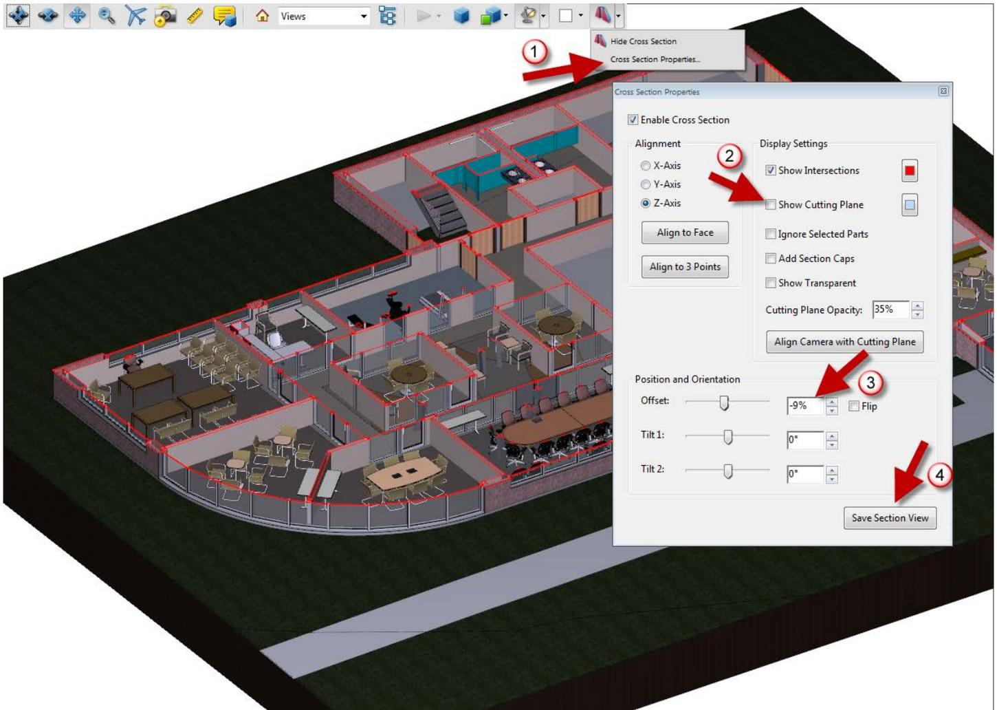
**Image 13:** Creating a cutaway view in the 3D PDF
